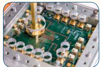
Integration photo of 45nm RF front-end IC with antenna and antenna interface.
